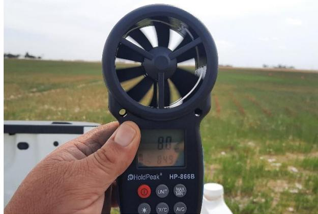
*Figure 19. Measuring wind and temperature at the trial site before making the treatment applications.*
