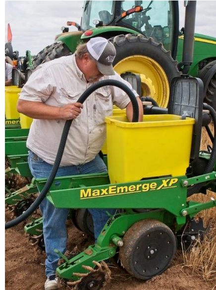
Figure 16. Vacuuming seed from seed boxes for replicated variety trial.
