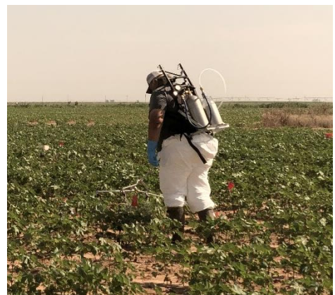
Figure 10. CO 2 backpack sprayer with auxin labeled tips making an application in cotton.
