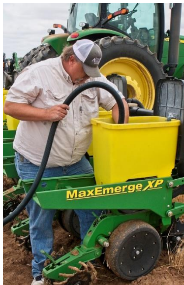
Figure 19. Vacuuming a planter and changing seed for a variety trial.
