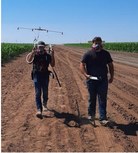
Figure 27. The CO2 backpack sprayer with boom attachment at work during the 2020 season.
